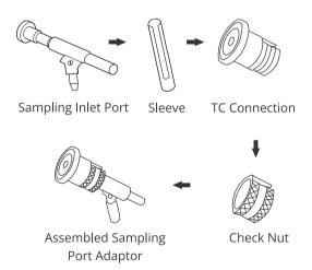
3. Attach the sampling syringe inlet port adaptor to the tri clover sampling port on the bioreactor/collection vessel with the help of a clamp.
