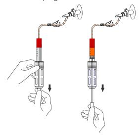
6. Pinch and cut to remove the filled sampling syringe.
