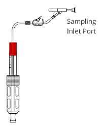
2. Fix the sampling port into the 25 mm ASESS sampling adaptor.
