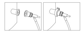
4. Sterilize the Bioreactor/vessel along with the aseptic sampling syringe inlet port by steaming in place the bioreactor vessel at 125°C for 30 minutes.
